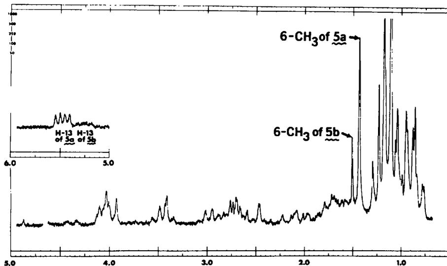
FIG 4. NMR spectrum of 5 in  $\text{CDCl}_3$  solution.
